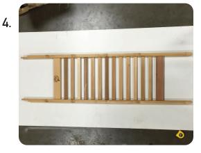
Using another person, push both posts toward each other until the Header, Slats & Footer are all the way in the grooved slots on both posts.
