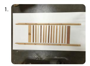
To start assembly of the sides of your VGA, lay out the posts, slats, header and footer on a flat surface as shown above. Make sure you keep the notched portion of the post to the outside. The flat side of all the slats MUST be facing up, the same way as the logo on the Header & the angled edges must be pointing up, towards top of the posts (the notched ends.)
