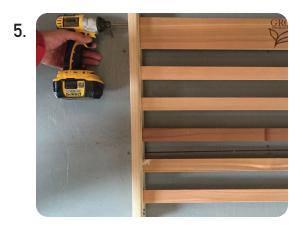
Using a screwdriver or power drill/driver, attach the Header, Slats & Footer to both posts, using the provided screws through the pre-drilled holes. REPEAT STEPS 1-5 FOR THE OTHER SIDE OF YOUR VGA.
